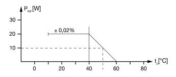
The max. load capacity with different ambient temperature as a function of the warm-up error can be taken from the load reduction curve. Example: Ambient temperature: max. 50°C; accepted  $\triangle$  R by temperature influence: max. 0.02 %; max. permissible load: 10 W.
