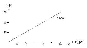
Cooling body temperature = ambient temperature + excessive temperature.
